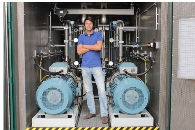
Booster Module with API610 pumps and pressurized buffer system for double mechanical sealing
